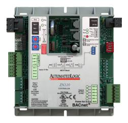
The ZN220 is a fully programmable, native BACnet Advanced Application Controller (AAC) designed for controlling a single zone in a building. It communicates on an EIA-485 LAN using BACnet over ARCnet or BACnet MS/TP communications and connects seamlessly to the WebCTRL<sup>®</sup> building automation system.
