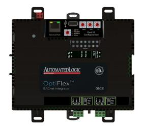
The Automated Logic® OptiFlex™ BACnet Integrator is an integral component of the WebCTRL® building automation system.
